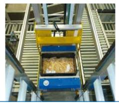
Transport Speed: up to 2.om/s Acceleration: 0.5 m/s<sup>2</sup>
